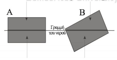
**Upward vertical force of buoyancy**
